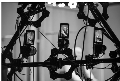
Fig. 1. Panasonic cameras used to capture multiple views of the interview.
